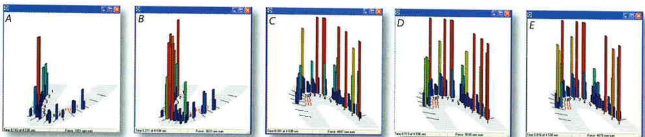
Fig. 2 Earliest tooth and implant prosthesis occlusal contacts (A) at .122 sec; The natural tooth depression into the periodontal ligament results in a force increase (B) at .189 sec; The end of intrasocket tooth movement with teeth at maximum force (C) at .281 sec; The first significant implant prosthesis force increase (D) at .396 sec; moderate forceful occlusal contacts on the implants (E) at .530 sec. Time delay is approximately .4 seconds.
